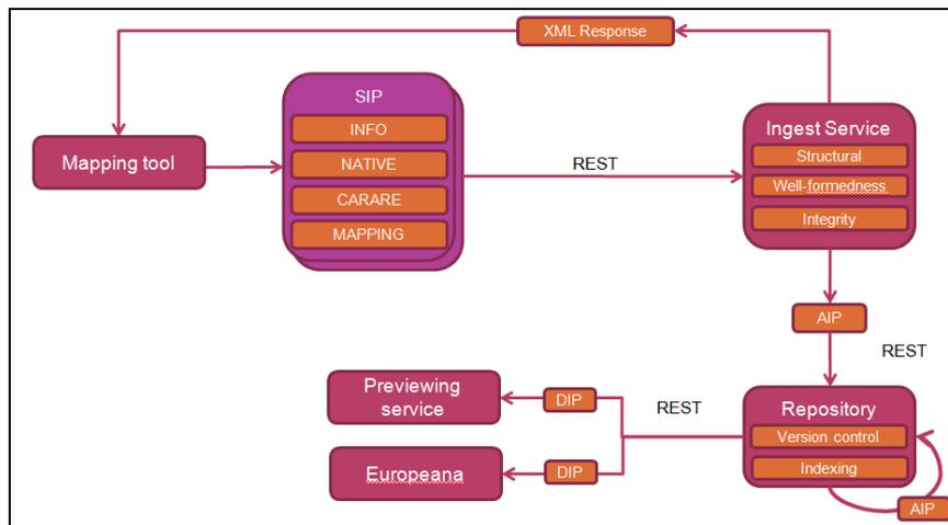
**Figure 7.2. Handling of the SIP packages.**
